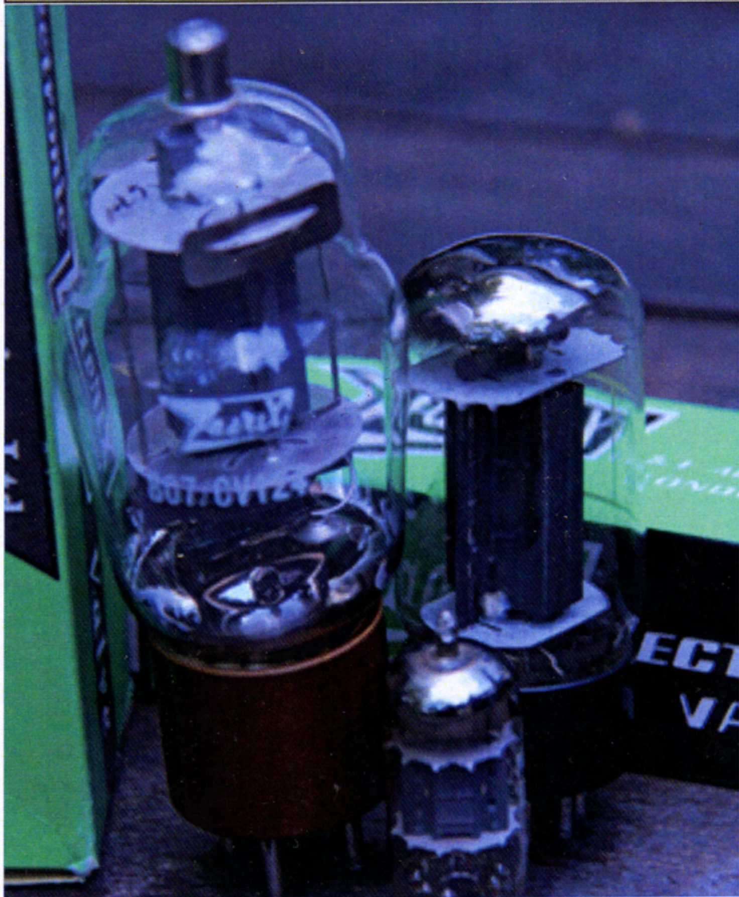
The valves from the original 10W transmitters: 807, 6L6 & ECC82
